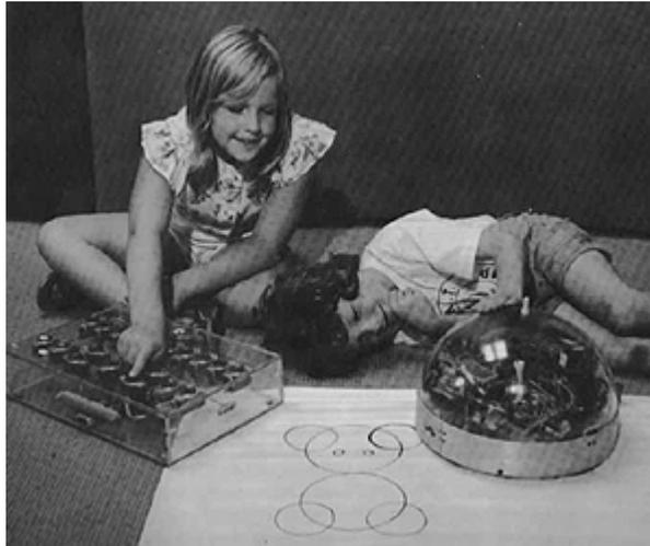
**Figure 4.** *Plotting a figure with a floor turtle (reprinted with permission from Taylor, 1980)*
