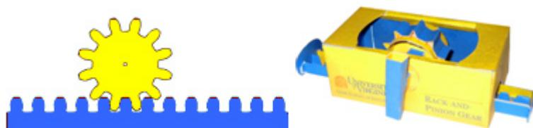
**Figure 5.** *Fabrication of a three-dimensional model derived from a two-dimensional drawing illustrating conversion of linear motion to rotary motion.*
